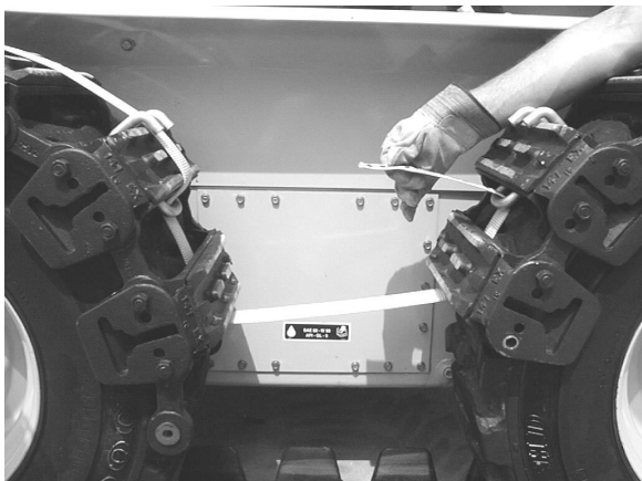
3: Pull strap across to right end of track, run strap under first pad of right end and through loop in binder bracket.
