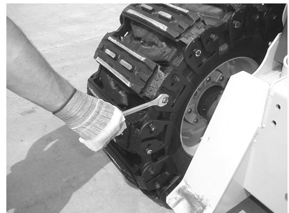
12: To ease in tightening bolts, move machine so bolts are at an accessible area. Torque bolts to 100-105 Ft. Lbs. Repeat for other side of skid steer.
