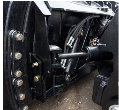
Relocated Tilt Cylinder Reduces Silage Build-up
