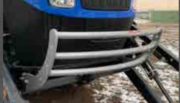
Standard Grille Guard to Protect Silage from Being Pushed into the Grille. (John Deere, Case IH, New Holland)
