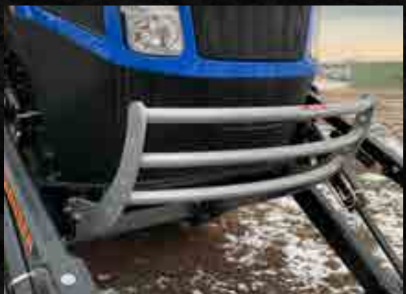
Standard Grille Guard to Protect Silage from Being Pushed into the Grille. (John Deere, Case IH, New Holland)
