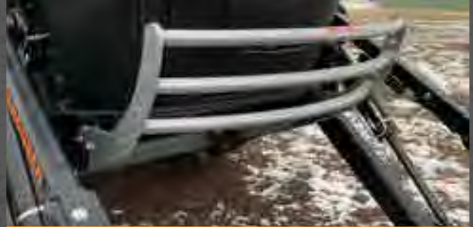
Standard Grille Guard to Protect Silage from Being Pushed into the Grille. (John Deere, Case IH, New Holland)
