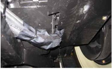
**2.** Run hoses up next to the fuel tank and over the transmission.
