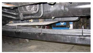
**1.** Run hoses through hose loops on undercarriage and push pole to the rear of the push pole.
