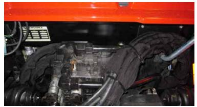
**4.** Run hoses up behind the valve and then back up over the valve from the right side between the cab and steel line. Plug hoses in. Verify that 3-point will not pinch any hoses.
