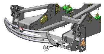
**25.** Install the grill guard to the front of the undercarriage with 3 - 3/4" x 2-1/2" bolts, 6 - 3/4" flat washers and 3 - 3/4" nuts on each side (14).
