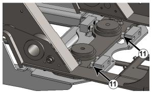
**22.** Unscrew the 1" x 2" bolts (#11) at the rear of the undercarriage until they are tight against the tractor frame. Torque the 1" bolts to 200 ft-lbs.
