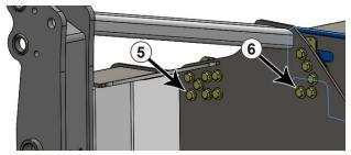
NOTE: Follow Steps #11-15 for the left side. After Step #15, tighten the bolts until they are snug. If necessary, add more shims until a gap of 1/16" or less is on the right side. Proceed with Step #11-14 for the right side.
