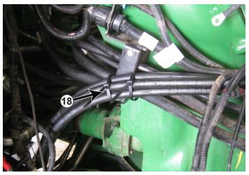
**5.** Route the hoses upward through the tractor. Staying away from the driveshaft by attaching the hoses to any other steel lines along the way. Attach to the tractor's hoses right by the hose bracket with zip ties (#18).
