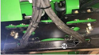
**2.** Route the hoses toward the center and attach to the undercarriage with a heavy zip tie (#16).
