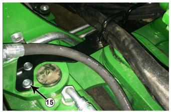
**27.** At the pivot area of the tractor, remove the bolts from the top plate that hold the cylinder pins and install the hose routing bracket along with the original plate and new 12mm flange bolts. Torque the 12mm bolts to the same specification that the tractor manufacturer recommends (#15).
