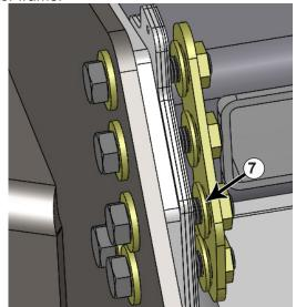
**15.** Place controller from Step # 13 on the bolts and thread a 3/4" flange nut on 4 of the top bolts from Step #14. Attach the nut plate to the bottom bolt and line up the top hex nuts to fit in the nut plate (#7). Note the orientation of the flange nuts.
