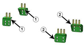
NOTE: The orientation of the left and right front brackets is important. Install the brackets as shown above.
