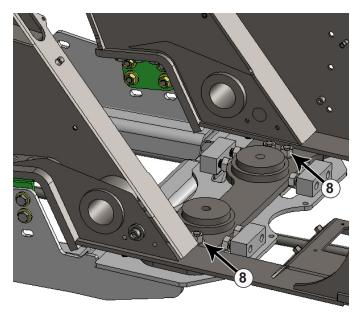
**16.** Attach the rear of the undercarriage vertically to the cross member on the tractor frame behind the rear axle with 4 - 7/8" x 3" bolts, 8 - 7/8" hardened flat washers, and 4 - 7/8" nuts (#8).
