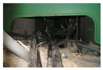
7. Route the hoses through the open cavity of the back section of the tractor. Secure hoses with zip ties where necessary to avoid rubbing and pinch areas. Plug the hoses into the open SCV's at the back of the tractor.
