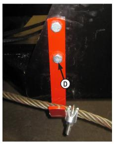
**4.** Install the original bracket to the side of the undercarriage with 2 - 3/4" x 2" bolts (PN: 16-20218) and 2 - 3/4" nuts (PN: 70-20607) **(D)**. Cable clamp is installed in Step #6.
