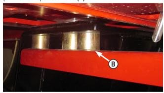
2. Install the front cable support bracket at the front of the undercarriage. Install with 3 spacers on each side in between the undercarriage and the bracket. Use 3 - 20mm x 120mm (PN: 16-2489) to install the bracket and undercarriage. Use the same washers and nuts that were used in the mounting instructions on Page 3 (B).
