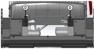
NOTE: If tow cable bracket was equipped, reinstall the bracket when installing the front 6 vertical bolts. See Page 5 for more hardware and installation information.
