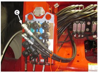
**5.** After installing the male couplers, plug each set into a set of rear SCV's **(C)**.
