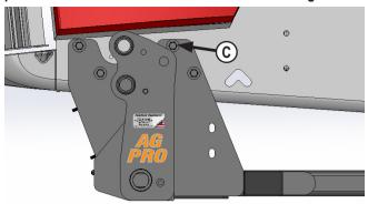
7. Install  $8 - 20mm \times 70mm$  bolts, 8 - 3/4" ID thick washers, shims if necessary, 8 - 3/4" flat washers, and 8 - 20mm nuts into the front side holes of the undercarriage and tractor frame **(C)**.
