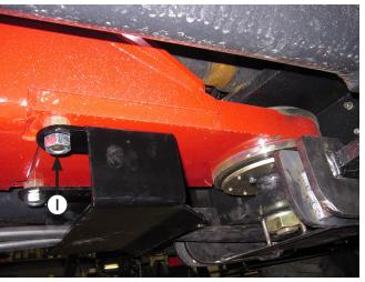
**22.** Attach the rear hose routing plate to the tractor frame behind the pivot point and before the drawbar. There will be 2 bolts sticking down. Attach with a 20mm nut on each side **(I)**. Make sure the lip of the plate is facing towards the front of the tractor.
