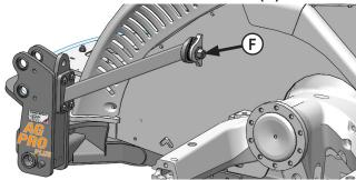
**14.** Attach the front upper support arms to the tractor with a 1-1/4" flat washer and 1-1/4" nut on each side **(F)**.
