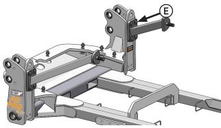
**13.** Attach the front upper support arms to the undercarriage with 4 - 3/4" x 2-1/2" bolts and 4 - 3/4" hardened flat washers on each side **(E)**.
