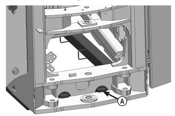
**5.** Lift the rear of the undercarriage and set the top plates on the tractor cross member **(A)**. Push the undercarriage back until the vertical push plates are firmly against the cross member.
