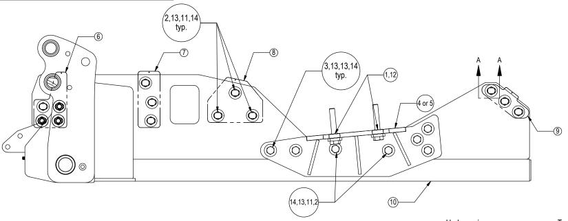
Note: Install all bolts before tightening.
