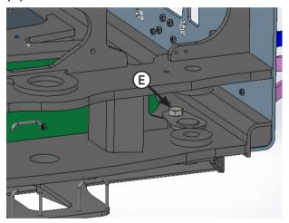
7. At the rear of the undercarriage, install 2 - Cat Tail Section washers, 2 - 1" x 5" bolts, and 2 - 1" nuts. Install the washer and the bolt from the top. Only hand tighten the nuts (E).
