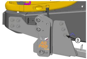
**6.** Install 6 - 1" x 4" bolts, 6 - 1" heavy washers, and 6 - 1" nuts in the rear holes of the side plates **(D)**.
