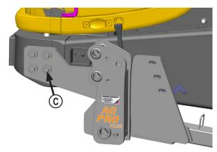
**5.** At the front of the tractor, install 8 - 24mm x 100mm bolts and 8 - 1" heavy washers **(C)**.
