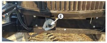
**5.** Move the original tow cable bracket to the right side and attach the tow cable with the original hardware **(E)**.
