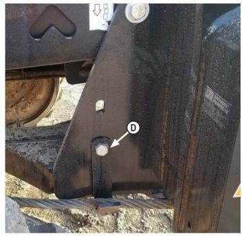
**4.** Attach modified tow cable bracket to the bottom slot on the right side of the undercarriage with original tow cable bracket hardware **(D)**.
