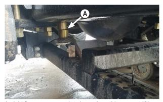
1. Add 2 spacers on each to lower the cable support (A).
