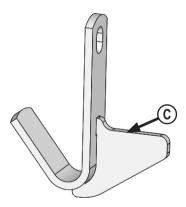
**3.** Tow cable bracket was removed in Step #1 on Page 2. Remove plate from tow cable bracket **(C)**.
