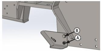
2. Remove hardware from top hole (B). Support bracket and move wire harness (A) to the top hole (B).
