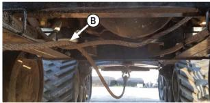
**2.** Route the cable underneath the undercarriage, then over the cable support and under the undercarriage on the right side **(B)**.
