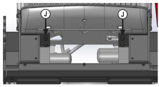
**13.** Attach the front of the undercarriage to the tractor frame with 6 - 20mm x 70mm bolts, 12 - 3/4" flat washers, and 6 - 20mm nuts. Insert the bolts from the bottom **(J)**.
