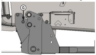
**10.** Install 8 - 20mm x 70mm bolts, 8 - 3/4" ID thick washers, shims if necessary, 8 - 3/4" flat washers, and 8 - 20mm nuts into the front side holes of the undercarriage and tractor frame **(G)**.
