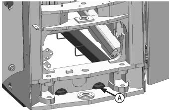
**5.** Lift the rear of the undercarriage and set the top plates on the tractor cross member **(A)**. Push the undercarriage back until the vertical push plates are firmly against the cross member.
