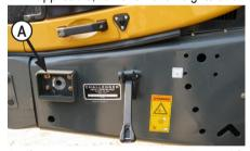
2. If necessary, remove the switch guard from the left side of the tractor (A). Reinstall the hardware without the switch guard.
