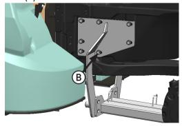
**4.** Attach the side brackets to the tractor with 14 - 20mm x 50mm bolts and 14 - 3/4" flat washers **(B)**.
