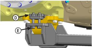
**7.** Place the clamp weld bracket on top of the drawbar bracket **(D)**.
