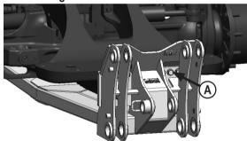
3. Lift the undercarriage and attach the front of the undercarriage to the tractor with 8 - 20mm x 70mm bolts and 8 - 3/4" flat washers (A).
