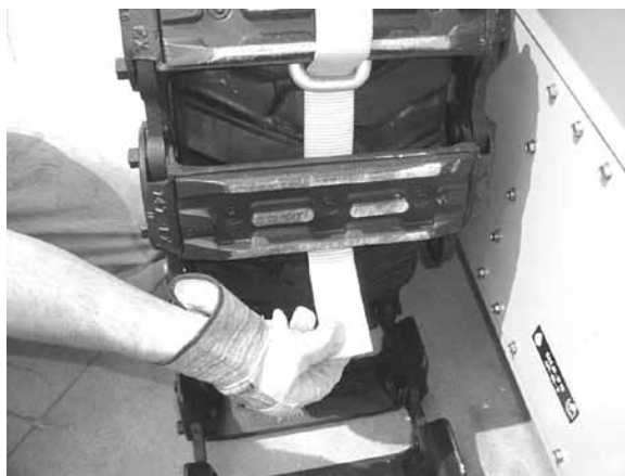
2: Thread strap through loop in binder bracket and under first pad from left end.
