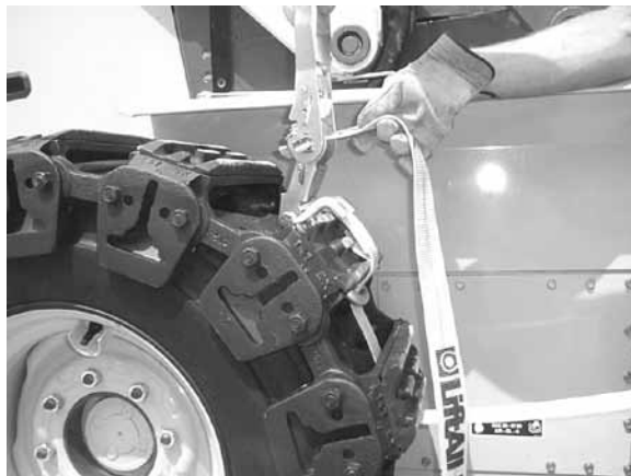
4: Slide end of strap through slot at center of ratchet assembly. Make sure there are not twists in strap.
