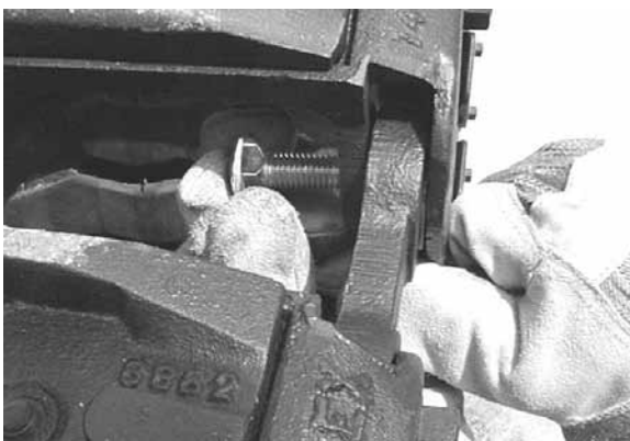
11: Insert bolts from inside of track. Put lock-nut on outside of track. Once both bolts are inserted, web binder and brackets may be removed.
