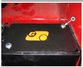
**37.** Place the valve cover over the valve and hoses as shown in the picture. Verify that the hoses are not being pinched.
