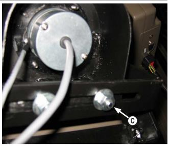
**4.** Attach the joystick mount (PN: 18-12038) to the joystick plate with 2 - 3/8" x 1" carriage bolts, 2 - 3/8" flat washers, and 2 - 3/8" nuts **(C)**.
