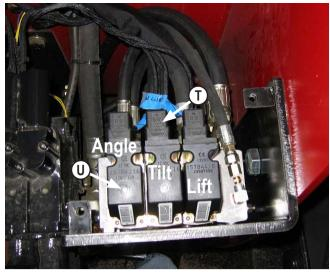
**31.** Guide the 3 cables and Dins from the wire harness out to the rear of the tractor **(T)**.
