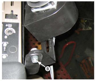
3. Attach the joystick plate (PN: 44-12032) to the joystick bracket with 2 - 3/8" x 1" carriage bolts, 2 - 3/8" flat washers, and 2 - 3/8" nuts **(B)**.
