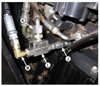
**16.** Install a JIC x Face Seal Swivel (PN: 31-12331-6-6) to the fitting that the hydraulic line was removed from. Also install a Female JIC Swivel x Male Pipe fitting (PN: 31-12332-6-4) onto the previous fitting (J).
