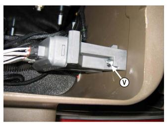
**36.** Drill a hole for a 1/4" bolt in the fuse compartment. Attach the wire harness to the compartment with a 1/4" bolt, 1/4" washer, and a 1/4" nut **(V)**.
