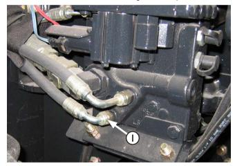
**15.** On the left side of the manifold valve, disconnect the bottom hydraulic line (I).
