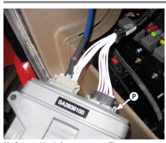
25. Set control box in fuse compartment (P).
