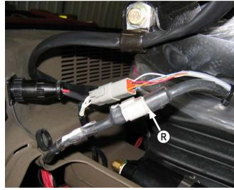
29. Connect the cable from the joystick to the wire harness (R).
