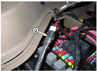
**26.** Connect the dozer angle extension cord to the wire harness **(Q)**. Run the cord through the hole in the floor of the fuse compartment.
