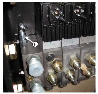
13. If fittings are not installed in the LS port on the control valve, install a straight -6-5 fitting (PN: 31-34033) and a  $90^{\circ}$  -6-6 fitting (PN: 31-34099) in the LS port (H).
