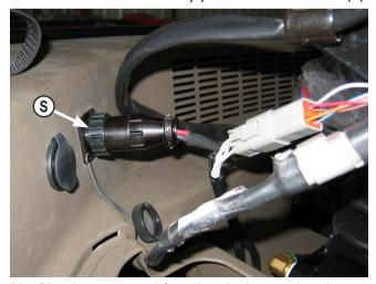
**30.** Plug the power cord from the wire harness into the port located behind and to the right of the operator's seat in the tractor cab (S).
