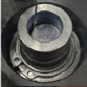
3. Inspect the seal and interior surfaces for contamination.
