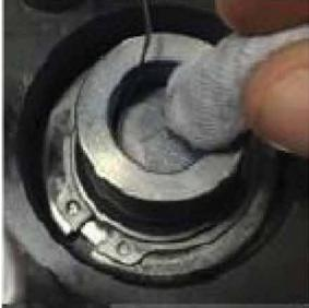
4. In case of contamination, carefully wipe surfaces with a soft cloth, or use compressed air to blow the contamination out. Do Not press hard on the seal as contamination can scratch the seal surface.
