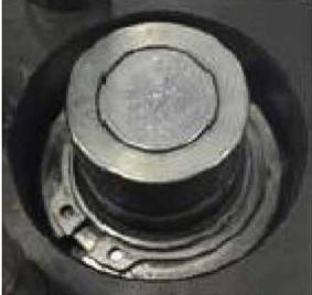
5. Using a non-marring tool, depress the valve face and remove the metal wire. Release the valve to the flush position.
