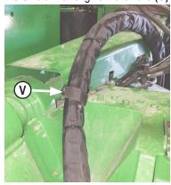
**6.** Use a velcro strap to group hoses together and attach to the PTO shield with 1 - 5/16" x 1" bolt and 1- 5/16" flat washer **(V)**.
