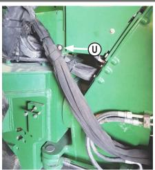
**5.** Route hoses up along right side of rear frame and group hoses together with a velcro strap. Attach velcro strap to the PTO shield with original hardware **(U)**.
