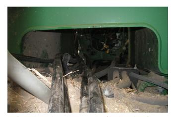
7. Route hoses through open cavity of back section of tractor. Secure hoses with zip ties where necessary to avoid rubbing and pinch areas. Plug hoses into open SCV's at back of tractor.
