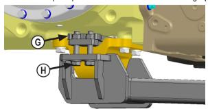
10. Place clamp weld bracket on top of drawbar bracket (G).
