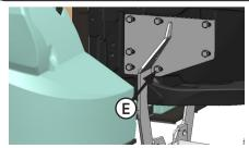
7. Attach side brackets to tractor with 14 - 20mm x 50mm bolts and 14 - 3/4" flat washers (E).
