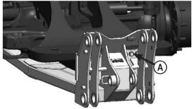
**3.** Lift the undercarriage and attach the front of the undercarriage to the tractor with 8 -  $20mm \times 70mm$  bolts and 8 - 3/4" flat washers (A).
