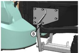
**4.** Attach the side brackets to the tractor with 14 - 20mm x 50mm bolts and 14 - 3/4" flat washers **(B)**.
