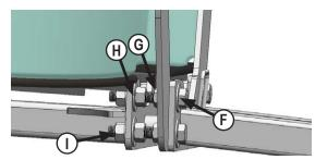
**9.** Install 4 - 1" x 8" bolts and 4 - 1" flat washers through the rear of the undercarriage and the side plates (**F**). Do Not push the bolts all the way through the push pole until the nuts are installed in the next step.
