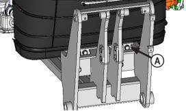
**3.** Lift undercarriage and attach front of undercarriage to tractor with 8 - 20mm x 70mm bolts and 8 - 3/4" flat washers (A).
