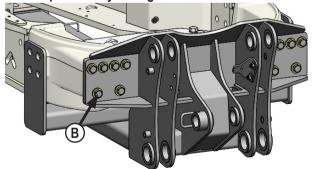
**4.** Raise undercarriage and attach front of undercarrige to tractor with 12 - 20mm x 70mm bolts and 12 - 3/4" flat washers **(B)**.
