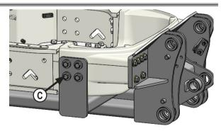
**5.** Attach side of undercarriage to tractor with 8 - 20mm x 50mm bolts and 8 - 3/4" x 3/8" thick heavy washers **(C)**.
