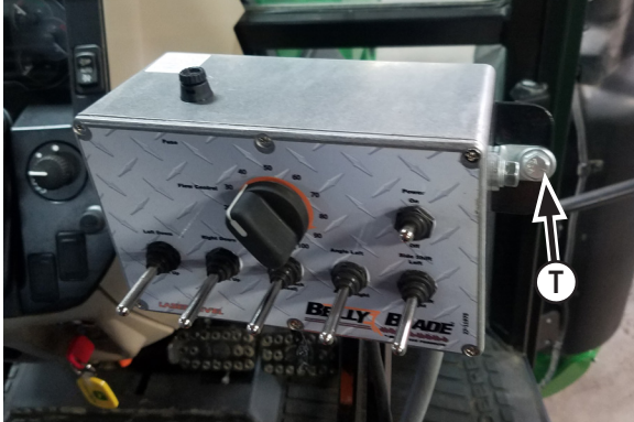
29. Attach controller to bracket with 2 - 5/16" x 1" bolts, 4 - 5/16" washers and 2 - 5/16" nyloc nuts (T).
