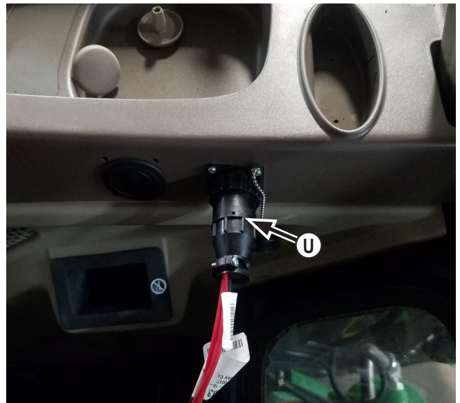
30. Attach the power cord from valve controller to auxiliary power socket (U).
