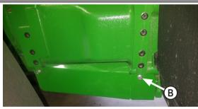
B. Remove cover on left side of tractor in front of fuel tank (B).
