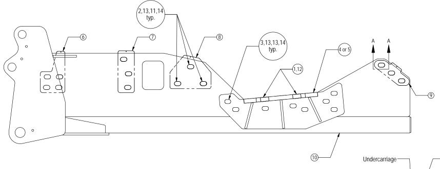
Note: Install all bolts before tightening.
