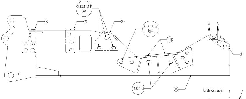
Note: Install all bolts before tightening.
