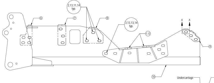
Note: Install all bolts before tightening.
