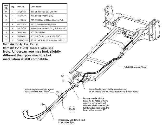
1. Attach the rear hose routing plate (PN: 44-17208) to the tractor frame behind the pivot point and before the drawbar. There will be 2 bolts sticking down. Attach with a 20mm nut (PN: 70-20872-10) on each side. Make sure the lip of the plate is facing towards the front of the tractor. See picture below for clarification.
