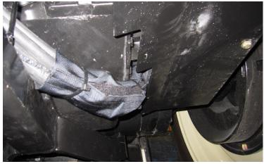
**2.** Run hoses up next to the fuel tank and over the transmission.
