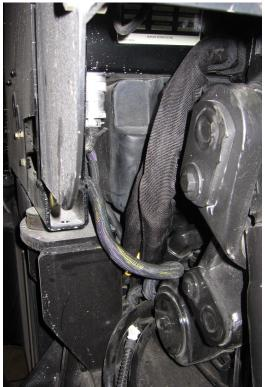
**3.** Run hoses above the transmission and out behind the 3-point on the left side.
