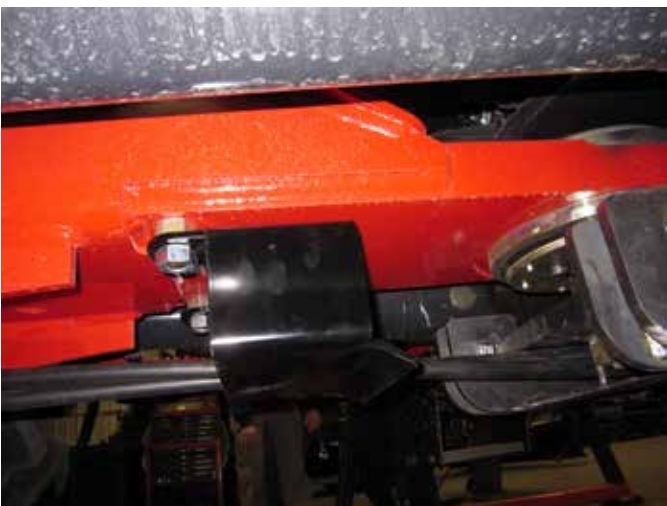
Hose Routing Plate attached with 20mm nuts. Picture doesn't show cordura on the hose but they should have cordura on them thru this pivot area of the tractor.
