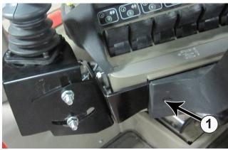
**2.** Attach the bolting bracket (PN: 18-16713) along with the cover or monitor mount to the front of the armrest with the original hardware from step #1. Put the bracket between the armrest and the cover or monitor mount (1).
