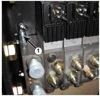
**13.** If fittings are not installed in the LS port on the control valve, install a straight -6-5 fitting (PN: 31-34033) and a 90° -6-6 fitting (PN: 31-34099) in the LS port (1).
