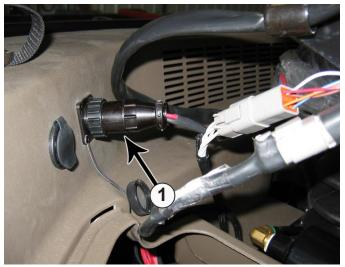
**27.** Plug the power cord from the wire harness into the port located behind and to the right of the operator's seat in the tractor cab (1).
