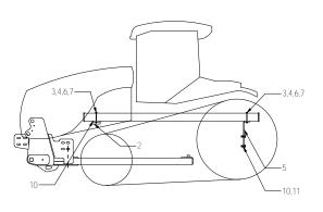
Note: Hose support bracket attached to tractor using front and rear step hardware.
