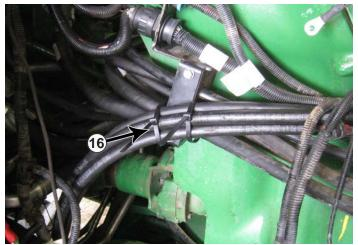
**5.** Route the hoses upward through the tractor. Staying away from the driveshaft by attaching the hoses to any other steel lines along the way. Attach to the tractor's hoses right by the hose bracket with zip ties (#16).
