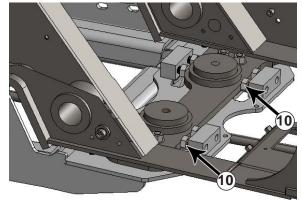
**21.** Unscrew the 1" x 2" bolts (#10) at the rear of the undercarriage until they are tight against the tractor frame. Torque the 1" bolts to 200 ft-lbs.
