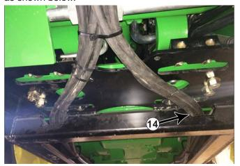
**2.** Route the hoses toward the center and attach to the undercarriage with a heavy zip tie (#14).
