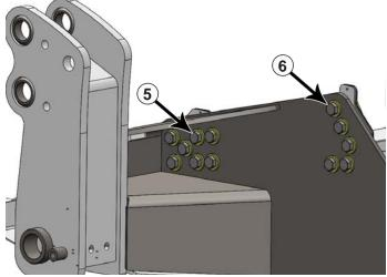
NOTE: Follow Steps #11-14 for the left side. After Step #14, tighten the bolts until they are snug. If necessary, add more shims on right side until a gap of 1/16" or less is on the right side. Proceed with Step #11-14 for the right side.
