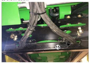
**2.** Route the hoses toward the center and attach to the undercarriage with a heavy zip tie (#15).
