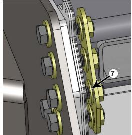
**14.** Thread a 3/4" flange nut on 4 of the top bolts from Step #13. Attach the nut plate to the bottom bolt and line up the top hex nuts to fit in the nut plate (#7). Note the orientation of the flange nuts.
