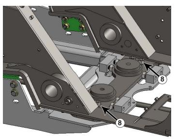
**15.** Attach the rear of the undercarriage vertically to the cross member on the tractor frame behind the rear axle with 4 - 7/8" x 3" bolts, 8 - 7/8" hardened flat washers, and 4 - 7/8" nuts (#8).
