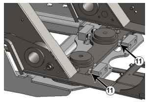
**21.** Unscrew the 1" x 2" bolts (#11) at the rear of the undercarriage until they are tight against the tractor frame. Torque the 1" bolts to 200 ft-lbs.
