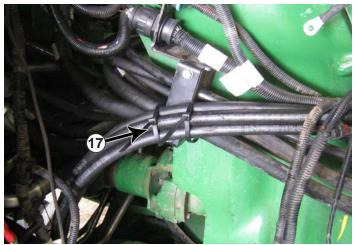
**5.** Route the hoses upward through the tractor. Staying away from the driveshaft by attaching the hoses to any other steel lines along the way. Attach to the tractor's hoses right by the hose bracket with zip ties (#17).
