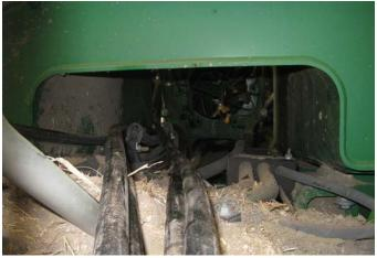
**6.** Continue the hoses through the open cavity of the back section of the tractor. Attach hoses where necessary to avoid rubbing and pinch areas. Plug the hoses into the open SCV's at the back of the tractor.
