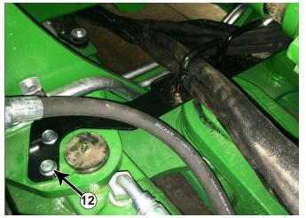
**22.** At the pivot area of the tractor, remove the bolts from the top plate that hold the cylinder pins and install the hose routing bracket along with the original plate and new 12mm flange bolts. Torque the 12mm bolts to the same specification that the tractor manufacturer recommends (#12).
