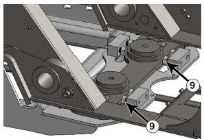
**19.** Unscrew the 1" x 2" bolts (#9) at the rear of the undercarriage until they are tight against the tractor frame. Torque the 1" bolts to 200 ft-lbs.
