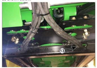
**2.** Route the hoses toward the center and attach to the undercarriage with a heavy zip tie (#13).
