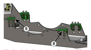
**14.** Attach the front and rear brackets (#8) to the inside of the undercarriage with a 3/4" x 2-1/4" bolt, 2 - hardened flat washers, and a 3/4" nut on each bolt.
