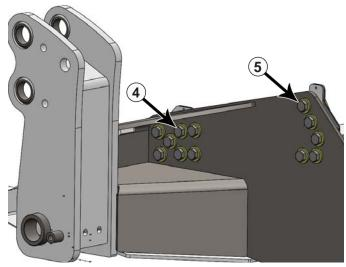
NOTE: Follow Steps #9-12 for the left side. After Step #12, tighten the bolts until they are snug. If necessary, add more shims on right side until a gap of 1/16" or less is on the right side. Proceed with Step #9-12 for the right side.
