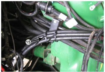
**5.** Route the hoses upward through the tractor. Staying away from the driveshaft by attaching the hoses to any other steel lines along the way. Attach to the tractor's hoses right by the hose bracket with zip ties (#15).
