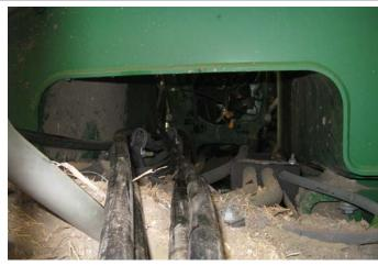
**6.** Continue the hoses through the open cavity of the back section of the tractor. Attach hoses where necessary to avoid rubbing and pinch areas. Plug the hoses into the open SCV's at the back of the tractor.
