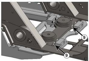
**19.** Unscrew the 1" x 2" bolts (#9) at the rear of the undercarriage until they are tight against the tractor frame. Torque the 1" bolts to 200 ft-lbs.
