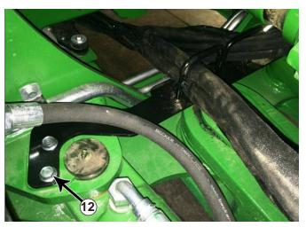
**22.** At the pivot area of the tractor, remove the bolts from the top plate that hold the cylinder pins and install the hose routing bracket along with the original plate and new 12mm flange bolts. Torque the 12mm bolts to the same specification that the tractor manufacturer recommends (#12).
