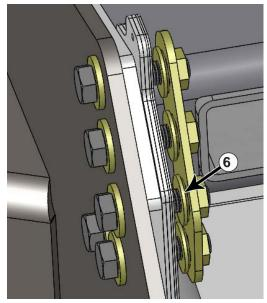
**12.** Thread a 3/4" flange nut on 4 of the top bolts from Step #11. Attach the nut plate to the bottom bolt and line up the top hex nuts to fit in the nut plate (#6). Note the orientation of the flange nuts.
