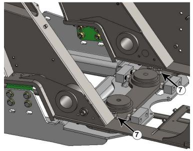
**13.** Attach the rear of the undercarriage vertically to the cross member on the tractor frame behind the rear axle with 4 - 7/8" x 3" bolts, 8 - 7/8" hardened flat washers, and 4 - 7/8" nuts (#7).
