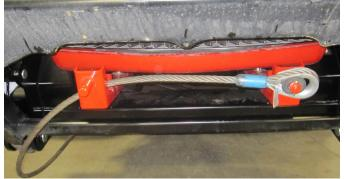
5. Finish routing the cable under the lift frame and up over the cable bracket. Attach to the bracket with the original hardware.
