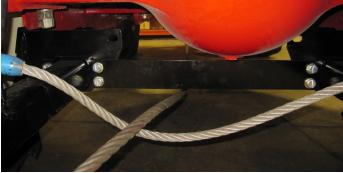
3. Route the cable underneath the undercarriage, then over the cable support and under the undercarriage on the right side.
