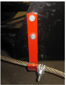
4. Install the original bracket to the side of the undercarriage with 2 - 3/4" x 2" bolts (PN: 16-20218) and 2 - 3/4" nuts (PN: 70-20607). Cable clamp is installed in Step #6.
