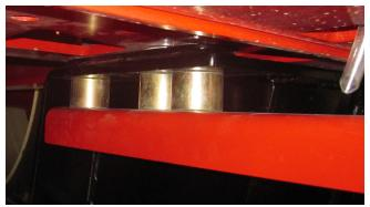
2. Install the front cable support bracket at the front of the undercarriage. Install with 3 spacers on each side in between the undercarriage and the bracket. Use 3 -20mm x 120mm (PN: 16-2489) to install the bracket and undercarriage. Use the same washers and nuts that were used in the mounting instructions on Pages 1.
