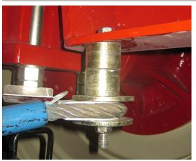
1. Add 2 spacers in between the cable holder and the tractor frame by the front tires. Use a 5/8" x 6" bolt (PN: 16-20200), 2 - 5/8" washers (PN: 57-20746) and a 5/8" top lock nut (PN: 70-20646) on each side.
