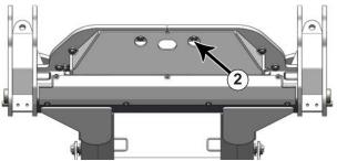
**6.** Lift the front of the undercarriage up and insert 8 - 20mm x 90mm bolts with a .375" thick washer on each bolt from the bottom through the front slots of the undercarriage that line up with the vertical holes on the tractor frame (2).
