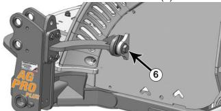
**14.** Attach the front upper support arms to the tractor with a 1-1/4" x 4-1/2" bolt and 1-1/4" flat washer on each side.
