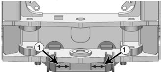
2. Send hoses through the bracket at the pivot point but stay on the outside of the rods that are by the center large nut on the tractor. The hoses should be between the rods and the inside plates of the bracket (1).
