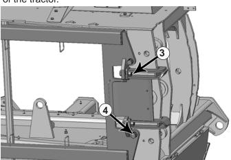
**8.** At the rear of the undercarriage and pivot area of the tractor, hook the rear hose routing bracket to the tractor frame and bolt to the rear of the undercarriage with 1" x 3" bolts, 1" hardened washers, and 1" nuts. The nut will fit between the plates on the brackets (3).
