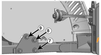
**15.** Install a side plate on each side of the undercarriage with 2 - 1" x 2" bolts and 2 - 1" ID x .375" thick washers (7).
