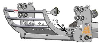
**24.** Install the grill guard to the front of the undercarriage with 3 - 3/4" x 1-3/4" bolts and 3 - 3/4" flat washers on each side (11).
