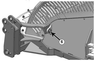
**14.** Attach the front upper support arms to the tractor with a 1-1/4" x 4-1/2" bolt, a 1-1/4" flat washer, and a 1-1/4" nut on each side.
