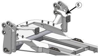
**13.** Attach the front upper support arms to the undercarriage with 2 - 1"  $\times 3-1/4$ " bolts, 2 - 1" hardened flat washers, and a 1" nut on the top bolt on each side (5).
