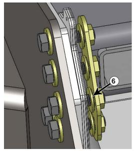
**12.** Thread a 3/4" flange nut on 4 of the top bolts from Step #11. Attach the nut plate to the bottom bolt and line up the top hex nuts to fit in the nut plate (#6). Note the orientation of the flange nuts.
