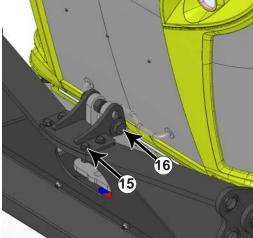
**19.** Attach the front top bracket to the front of the undercarriage with 4 - 3/4" x 2-1/2" bolts (PN: 16-20220), 8 - 3/4" hardened flat washers (PN: 57-20757) and 4 - 3/4" nuts (PN: 70-20607) (#15). **20.** Attach the front top bracket to the
