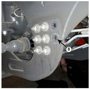
**8.** In front of the rear axle, remove the front two bolts on each side (#8) as shown above. The washers will be reused in Step #12.
