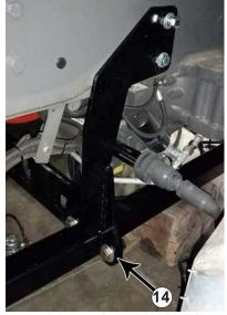
**18.** Attach the side brackets to the front and the rear undercarriage weldments with 1" x 3" bolts (PN: 16-20562) and a 1" flat washer on each bolt (PN: 57-20749). Once all the bolts are through the holes, attach with a 1" flat washer and a 1" nut" (PN: 70-20599) on each bolt (#14).
