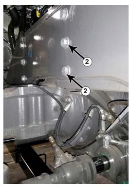
**4.** Behind the front axle, remove the bottom 2 bolts from each side of the tractor. You will reuse the washers from each bolt and the nuts from the bottom bolt on each side (#2)
