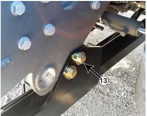
**17.** In front of the front axle, insert a 7/8" x 3-1/2" bolt (PN: 16-20544) with a 7/8" heavy washer (PN: 57-3681) into each slot of the undercarriage and into the tractor frame on each side. Then on the inside attach with a 7/8" heavy washer (PN: 57-3681) and a 7/8" nut (PN: 70-20598) (#13).
