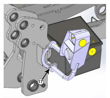
**21.** Attach the light brackets to the front of the undercarriage with 3 - 3/8" x 1-1/4" carriage bolts (PN: 16-21065) and a 3/8" flange nut (PN: 70-20622) on each bolt. Also use one of the original light bracket bolts, washer and nut (#17). Reconnect the light wire harness. Torque the 3/8" hardware to 33 ft-lbs.
