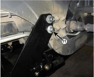
**12.** Attach the rear weldment to the tractor holes with 24mm x 100mm bolts (PN: 16-2486) and the washers that were removed in Step #8 and 24mm nuts (PN: 70-20874) (#11).
