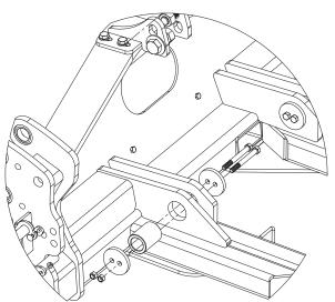
**16.** Insert the front pin (PN: 43-18531) into the front side of the undercarriage and into the frame of the tractor. The bolts will need to be inserted from the inside. Hold the pin in place by using 2 - 5/8" x 6" bolts (PN: 16-20200), 2 clamp plates (PN: 44-18003) and 2 - 5/8" nuts (PN: 70-20646) on each side.
