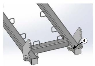
6. Install 4 - 1" x 3 bolts (PN: 16-20562) in the threaded boxes on the rear undercarriage weldment. The bolt heads need to be towards the back (#4). Turn the bolts all the way in for installation. The bolts will be adjusted in Step #28. **NOTE:** A full diagram of the assembly with the full list of parts is on Page 8.
