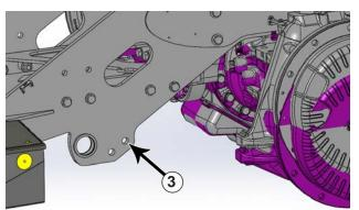
**5.** If applicable, remove 2 bolts in front of the front axle from each side of the tractor (#3).
