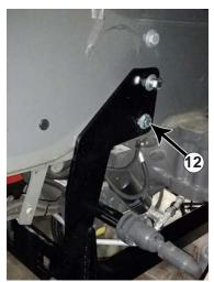
**13.** Behind the front axle, attach the side brackets to the tractor with 2 - 20mm x 110mm bolt (PN: 16-20150110) and a washer that was removed in Step #4 on each bolt. On the inside attach with a washer and nut that was removed in Step #4 on the bottom bolt on each side (#12).
