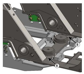
**15.** Attach the rear of the undercarriage vertically to the cross member on the tractor frame behind the rear axle with 4 - 7/8" x 3" bolts, 8 - 7/8" hardened flat washers, and 4 - 7/8" nuts (#8).
