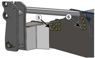
NOTE: Follow Steps #11-14 for the left side. After Step #14, tighten the bolts until they are snug. If necessary, add more shims until a gap of 1/16" or less is on the right side. Proceed with Step #11-14 for the right side.
