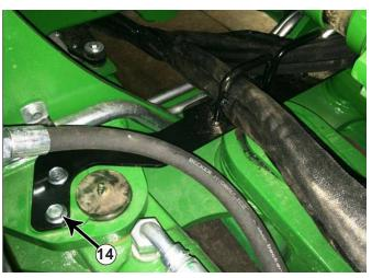
**24.** At the pivot area of the tractor, remove the bolts from the top plate that hold the cylinder pins and install the hose routing bracket along with the original plate and new 12mm flange bolts. Torque the 12mm bolts to the same specification that the tractor manufacturer recommends (#14).
