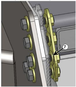
**14.** Thread a 3/4" flange nut on 4 of the top bolts from Step #13. Attach the nut plate to the bottom bolt and line up the top hex nuts to fit in the nut plate (#7). Note the orientation of the flange nuts.
