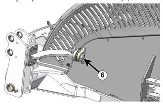
**14.** Attach the front upper support arms to the tractor with a 1-1/4" x 4-1/2" bolt, a 1-1/4" flat washer, and a 1-1/4" nut on each side (6).
