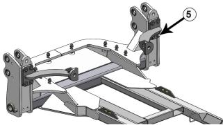
**13.** Attach the front upper support arms to the undercarriage with 4 - 3/4" x 2-1/2" bolts and 4 - 3/4" heavy duty flat washers on each side (5).
