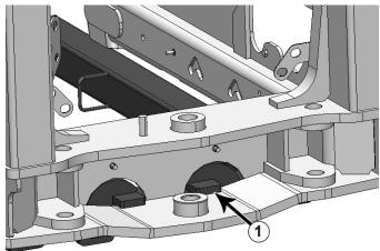
**5.** Lift the rear of the undercarriage up and set the top plates at the rear of the undercarriage on the tractor cross member (1). Push the undercarriage back until the vertical push plates are firmly against the cross member.
