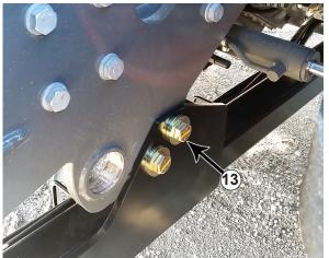
**17.** In front of the front axle, insert a  $7/8^{\circ} \times 3-1/2^{\circ}$  bolt with a  $7/8^{\circ}$  heavy washer into each slot of the undercarriage and into the tractor frame on each side. Then on the inside attach with a  $7/8^{\circ}$  heavy washer and a  $7/8^{\circ}$  nut (#13).
