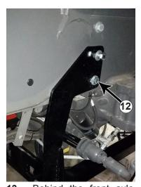
**13.** Behind the front axle, attach the side brackets to the tractor with 2 - 20mm x 110mm bolt and a washer that was removed in Step #4 on each bolt. On the inside attach with a washer and nut that was removed in Step #4 on the bottom bolt on each side (#12).
