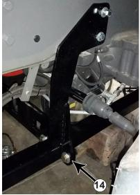
**18.** Attach the side brackets to the front and the rear undercarriage weldments with  $1^{\circ} \times 3^{\circ}$  bolts and a 1° flat washer on each bolt. Once all the bolts are through the holes, attach with a 1° flat washer and a 1° nut° on each bolt (#14).
