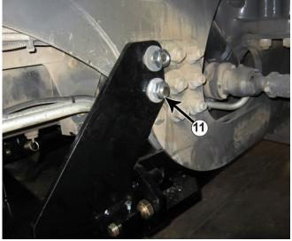
**12.** Attach the rear weldment to the tractor holes with 24mm x 100mm bolts and the washers that were removed in Step #8 and 24mm nuts (#11).
