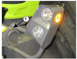
**3.** Disconnect the wire harness from the lights in front of the front tires. Remove the carriage bolts (#1) and remove the bracket and lights from the tractor. They will be reinstalled to the undercarriage in a later step.
