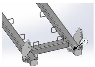
**6.** Install 4 - 1" x 3 bolts in the threaded boxes on the rear undercarriage weldment. The bolt heads need to be towards the back (#4). Turn the bolts all the way in for installation. The bolts will be adjusted in Step #28.
