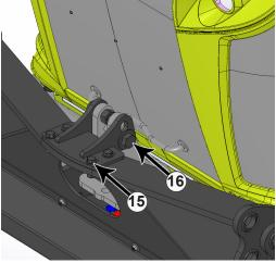
**19.** Attach the front top bracket to the front of the undercarriage with 4 - 3/4" x 2-1/2" bolts, 8 - 3/4" hardened flat washers and 4 - 3/4" nuts (#15).
