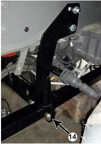
**18.** Attach the side brackets to the front and the rear undercarriage weldments with 1" x 3" bolts and a 1" flat washer on each bolt. Once all the bolts are through the holes, attach with a 1" flat washer and a 1" nut" on each bolt (#14).
