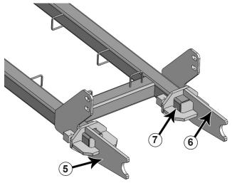
7. Put the rear brackets (PN: 18-17996-R,L) on the rear undercarriage weldment (PN: 54-17990) (#5). The orientation of the bracket should be as shown in the photo. The flat edge of the plate should be on top (#6) and the larger opening for the tube on the inside (#7).
