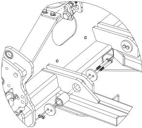
**16.** Insert the front pin (PN: 43-18531) into the front side of the undercarriage and into the frame of the tractor. The bolts will need to be inserted from the inside. Hold the pin in place by using 2 - 5/8" x 6" bolts, 2 clamp plates and 2 - 5/8" nuts on each side.
