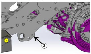
**5.** If applicable, remove 2 bolts in front of the front axle from each side of the tractor (#3).
