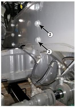
**4.** Behind the front axle, remove the bottom 2 bolts from each side of the tractor. You will reuse the washers from each bolt (#2).
