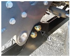
**17.** In front of the front axle, insert a 7/8" x 3-1/2" bolt with a 7/8" heavy washer into each slot of the undercarriage and into the tractor frame on each side. Then on the inside attach with a 7/8" heavy washer and a 7/8" nut (#13).
