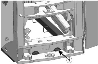
**5.** Lift the rear of the undercarriage and set the top plates on the tractor cross member (1). Push the undercarriage back until the vertical push plates are firmly against the cross member.
