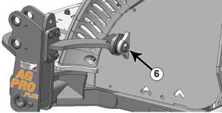
**14.** Attach the front upper support arms to the tractor with a 1-1/4" x 4-1/2" bolt and 1-1/4" flat washer on each side.
