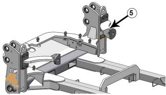
**13.** Attach the front upper support arms to the undercarriage with 4 - 3/4" x 2-1/2" bolts and 4 - 3/4" hardened flat washers on each side (5).
