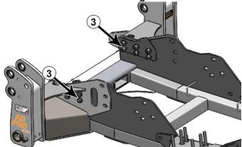
NOTE: Follow Steps #7-12 for the left side. After Step #12, tighten the bolts until they are snug. If necessary, add more shims on right side until a gap of 1/16" or less is on the right side. Proceed with Step #7-12 for the right side.
