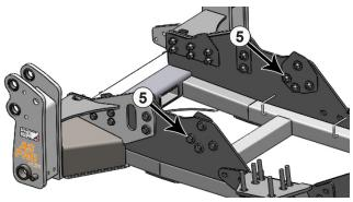
**9.** Install 4 - 7/8 " x 2-1/2" bolts with a 7/8" ID thick washer (#5) through the 3rd batch of holes on each side of the U/C, shims if necessary, and the tractor frame.
