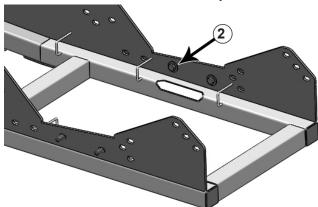
**5.** Install 2 - 7/8" x 2-1/2" bolts with a heavy duty flat washer (#2) on each bolt from the inside of the undercariage into the 2 center bolting locations for the axle brackets.
