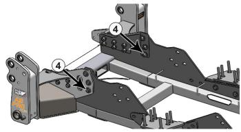
**8.** Install 3 - 7/8 " x 3" bolts with a 7/8" ID thick washer (#4) through the 2nd batch holes on each side of the U/C, shims if necessary, and the tractor frame.
